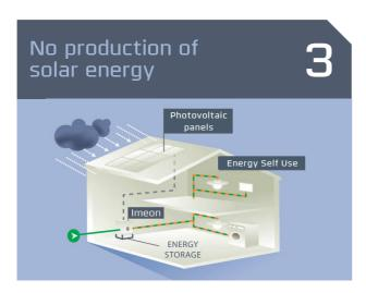
The batteries feed the domestic consumption needs. When needed, an eventual compliment of electricity is supplied by the public grid.
