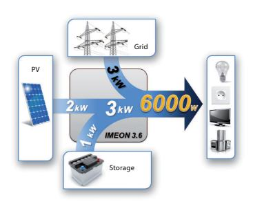
2kW of solar energy, 1kW of battery power and 3 kW from the grid for a total draw and output of 6kW . Thus, the installer does not need to modify the domestic electrical panel if it can provide energy less than or equal to 6kW.
