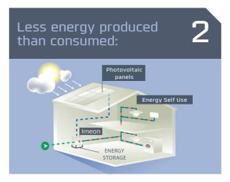
Solar power feeds a part of the consumption needs. The batteries and the public grid provide the remaining complimentary power.
