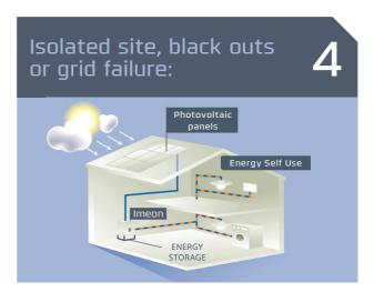
The solar installation feeds the domestic consumption needs first and charges batteries. The batteries then provide the eventual complimentary power.
