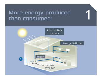
Solar energy power feeds consumption needs and simultaneously charges the batteries. An eventual surplus of solar power is then injected to the grid.
