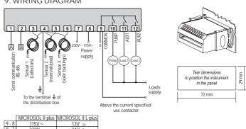
Note: The sensor cable length can be increased by the user until 200 meters using PP 2 x 24 AWG cable
