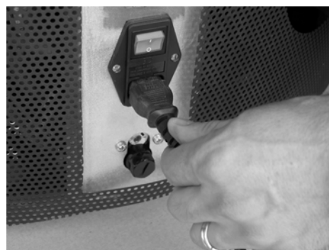
Figure 17 – Disconnect the stove from the electrical mains
