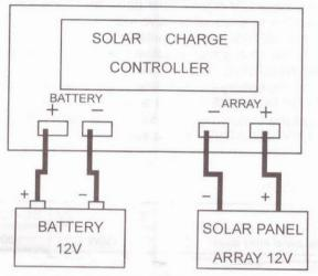
24V system: 24V solar panel, 24V battery and 24V/12V selection switch must be set to 24V.
